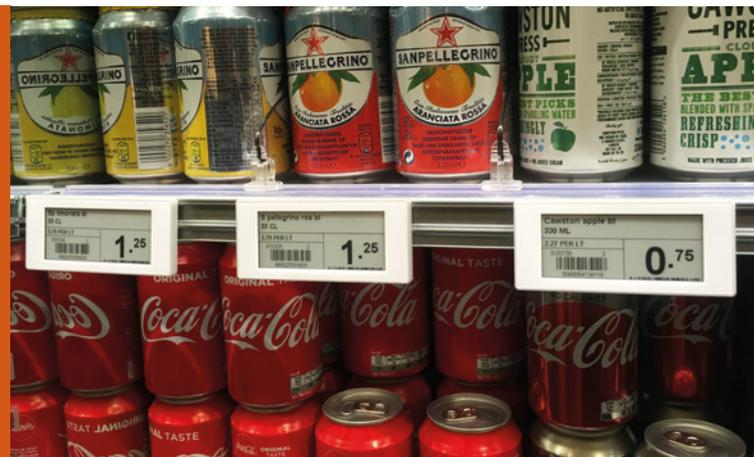
But Opticon's PE-range has more functionalities; when you tap on the ESL the LEDs provide a visual indicator and blink green whilst also giving a sound feedback that there was a successful transaction. In case there is a fault, the LEDs will blink red and give a different sound. If you take two products of the shelf, then the customer simply taps twice on the ESL, or when he decides to place the article back on the shelf the card/phone needs to be held
