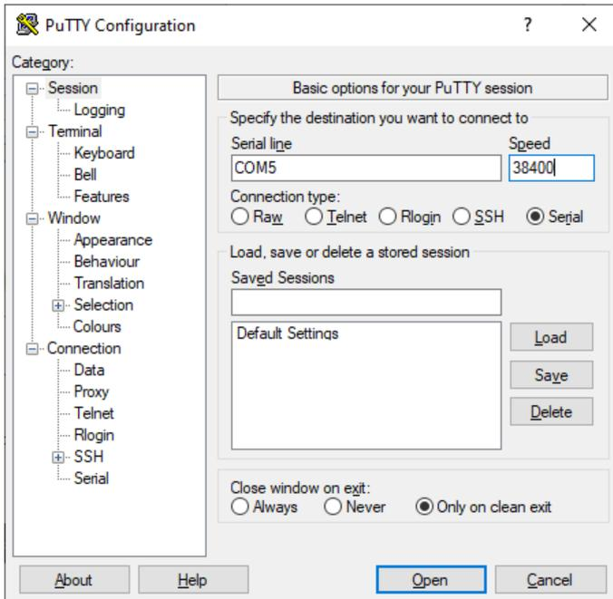
**Figure 174: PuTTY configuration for COM access**
