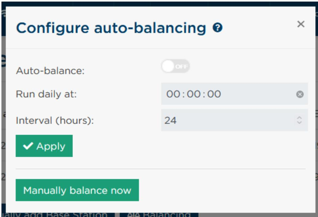
Figure 20: Balancing option window
