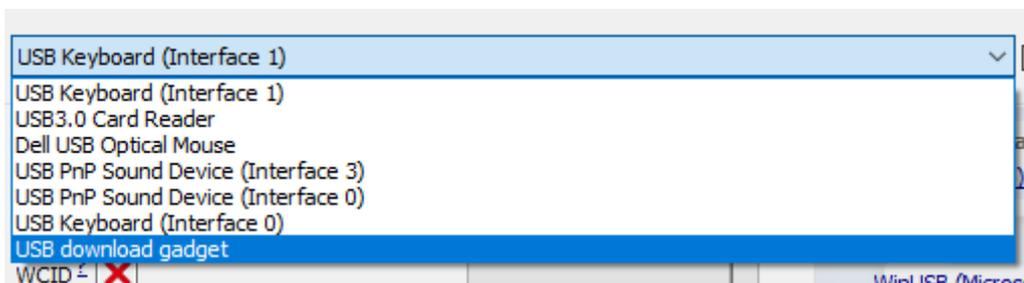
Figure 148: Enumerated USB devices with EBS-50 connected
