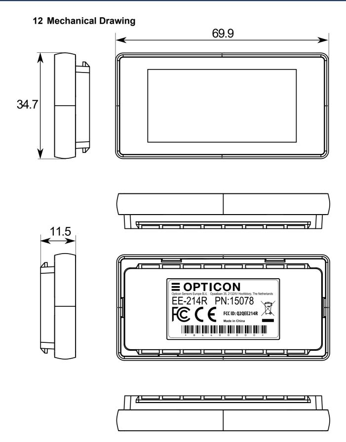
Figure 8: Mechanical drawing
