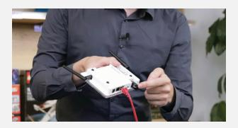
Use the EBS Power Supply to provide the Base Station with 6V power. You can use the EBS Ethernet cable to connect the Base Station to your existing network.
