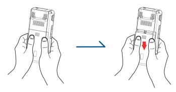
2) Press forcefully when inserting the battery.
