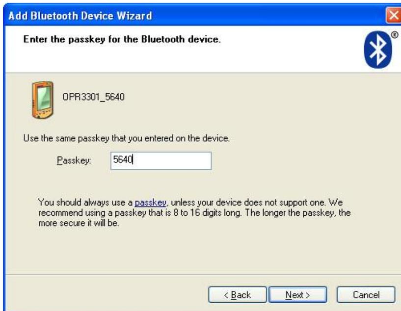
*Example of a request on a Windows device to enter a PIN-code (passkey)*
