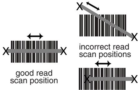
When reading a small bar code, decrease the distance between the terminal and the bar code. For larger bar codes, position the terminal so that the bar code fits into the laser beam. When reading a very high density bar code, decrease the distance between the terminal and the bar code. For a low density bar code, increase the distance between the terminal and bar code.
