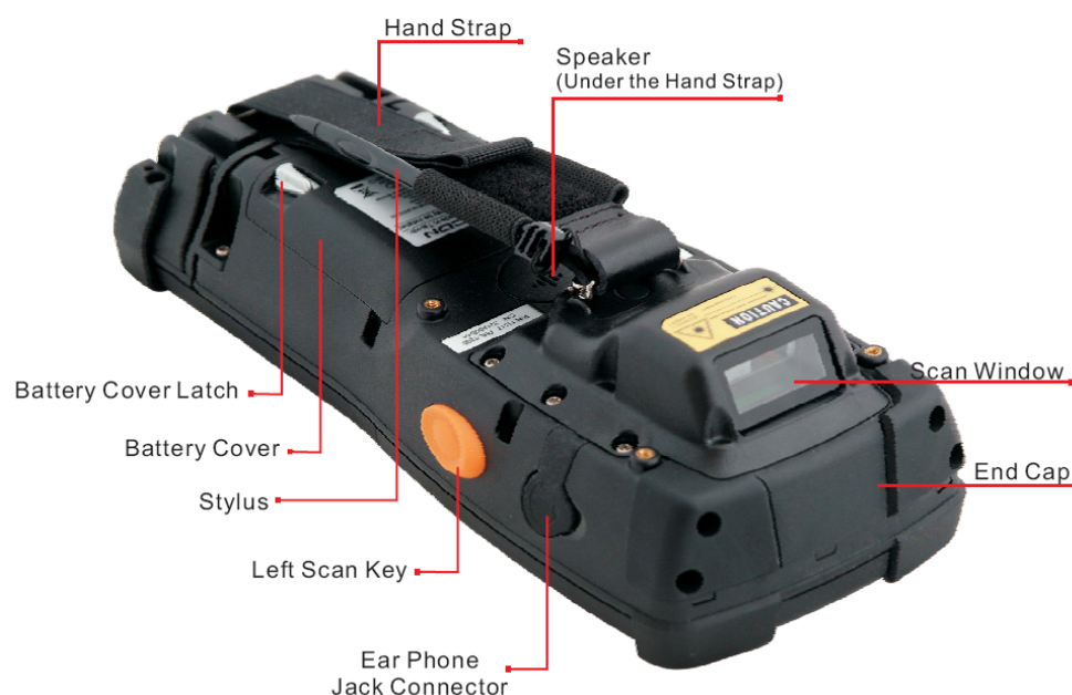
Figure 2-6 PHL-7200 rear view
