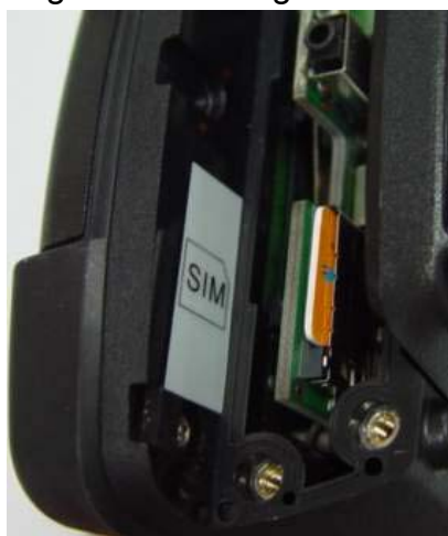
Figure 6-2 Insert SIM card
