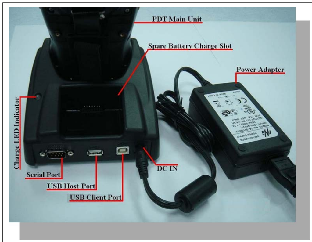
Figure 2-12 Charging with IRU-7000 cradle
