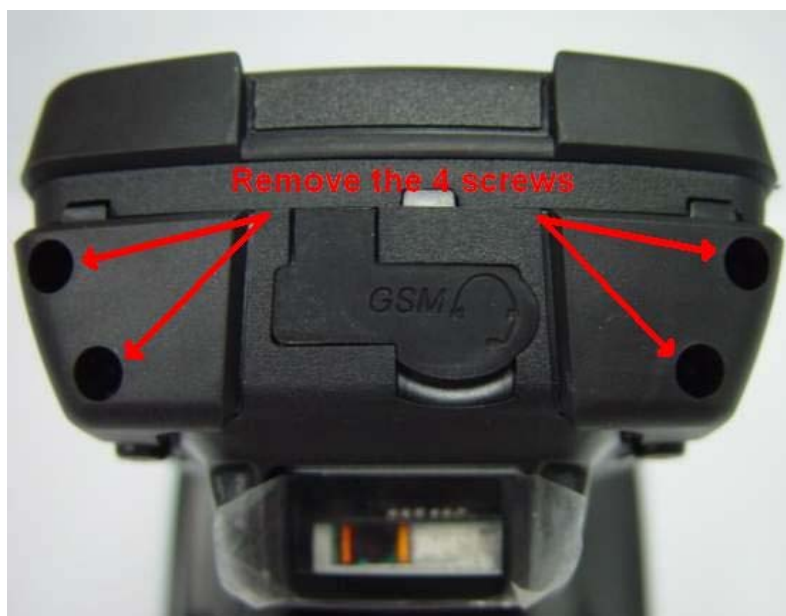
Figure 6-1 Remove screws from End Cap
