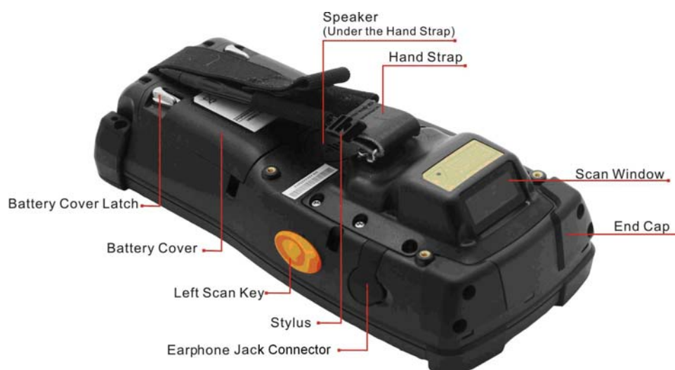
Figure 2-4 PHL-7100 rear view
