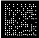
DataMatrix in negative dot print
